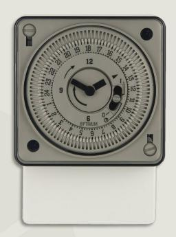
OP-TS111.1 IS A CAPTIVE-TAPPET 24-HOUR TIME SWITCH. EACH TAPPET OPERATES FOR 15 MINUTES. THE TIMER IS SUITABLE FOR SURFACE, PANEL AND DIN-RAIL MOUNTING. THE 24 HOUR DIAL CONTROLS A VOLT-FREE CHANGEOVER SWITCH, WITH A RESISTIVE RATING OF 16 AMPERES.
