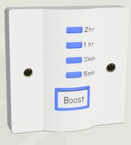
OP-EBT2 IS A ONE-BUTTON BOOST TIMER. THERE ARE FOUR PRE-SET TIMED OUTPUTS. SUITABLE FOR INSTALLATION ON A SURFACE OR IN-WALL PATTRESS BOX. THE ELECTRONIC TIMER CONTROLS AN INTERNALLY LINKED OUTPUT RELAY, WITH A RESISTIVE RATING OF 16 AMPS. AN EARTH PARK TERMINAL IS PROVIDED. SURFACE-RUN CORD OUTLET WITH CABLE RESTRAINT. PRESS UP TO 4x TO SELECT BOOST OUTPUT, PRESS AGAIN TO CANCEL.
